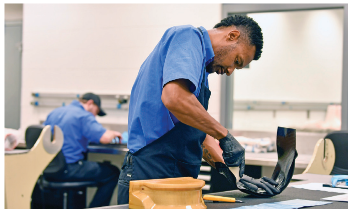
This carbon fiber part was made using the 3D printed lay-up tool.
