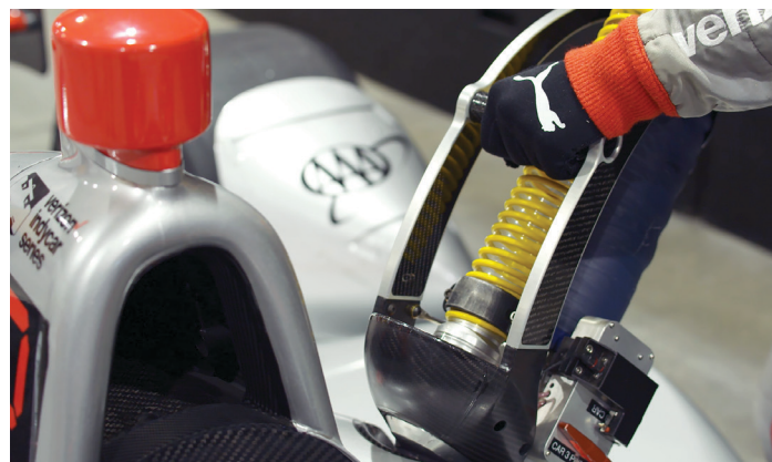
3D printed composite tooling was critical to meeting the deadline for producing the new fueling probe handle.
